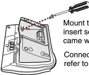
Mount the stand as shown and insert screw. Use the screw that came with your telephone.
